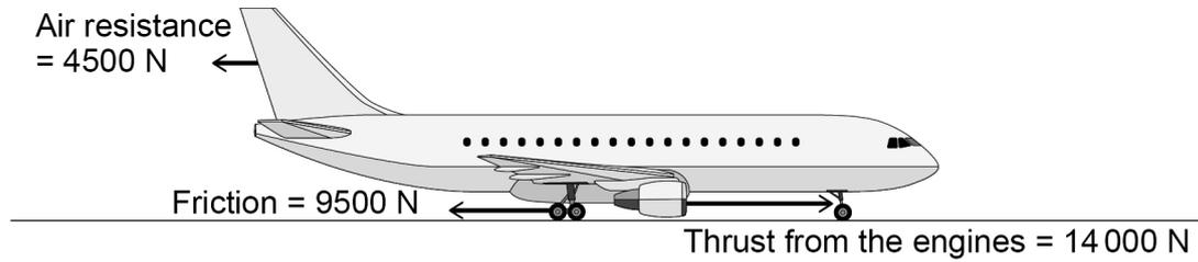
**0 2 . 2** Determine the magnitude of the resultant horizontal force on the aeroplane.
