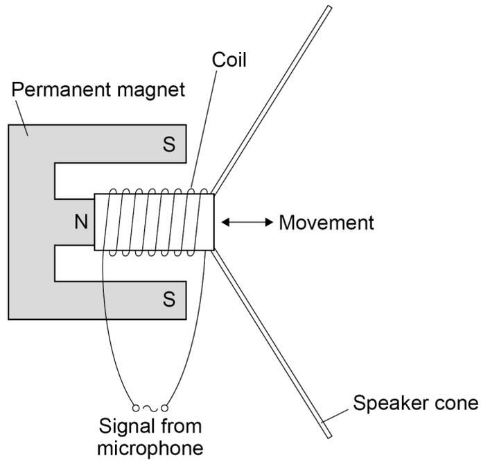
A current in the coil of the loudspeaker causes the coil to move.
