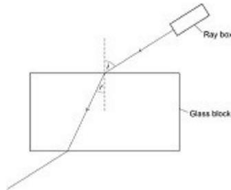
both rays in the air should be parallel
